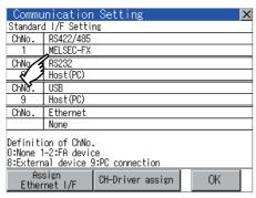
Touch the driver display BOX of the communication parameter to be set in the [Communication setting] screen.
