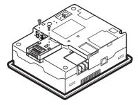
Fix the connection conversion adapter to the GOT using the provided M3 tapping screws. Tightening torque: 0.3 to 0.6 N•m
