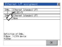
Touch the driver display BOX of the communication parameter to be set in Ethernet I/F assignment.
