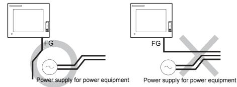
Good: Wiring the ground cable away from the power cable
