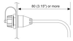
(5) Insert the USB plug part of the tip of the panel-mounted USB port extension securely to the USB port of the GOT.
