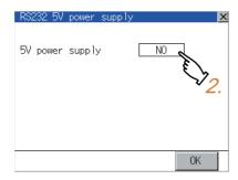
2. Touch the setting item of [5V power supply] when using the RS-232/485 conversion adaptor. The setting content is changed by touching. (YES NO)
