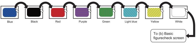
Touching the upper right part of the screen at the final color (white screen) displays the following (b) Basic figure check screen.
