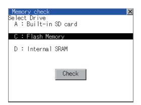
1. Select a drive to check in the Select Drive screen in Memory check and touch [Check] button.
