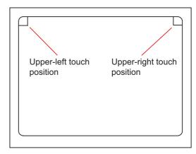
The installed font data is displayed by touching the upper right part of the screen.
