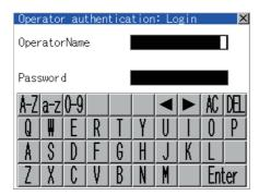
Log into the GOT with the operator name corresponding to the password to be changed on the Main Menu screen for the utility.
