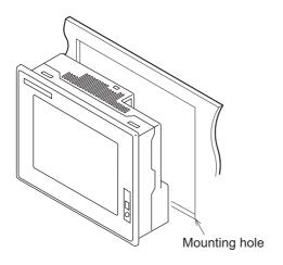
Inserting into the panel face Insert the GOT from the front side of the panel.
