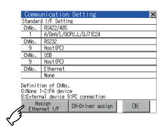
1. Touch the [Assign Ethernet I/F] button in [Communication Setting].
