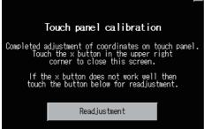
Touching the button displayed on the upper right returns the screen to the previous screen. When the precise touch could not be made, touch the [Readjustment] button to make the setting from again.
