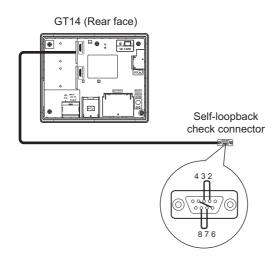
1. For preparation for the self-loopback communication check, insert the connector for self-loopback check (Customer purchased) shown in the diagram left in the RS-232 interface.
