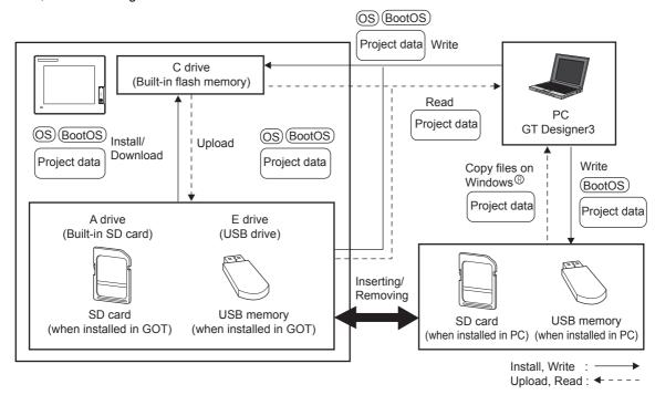
The data of the Flash Memory (Project data, etc.) can be saved even if the battery voltage becomes low.
