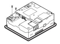
Fix the RS-232/485 signal conversion adaptor to the GOT using the provided M3 tapping screws.
