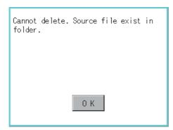
When it cannot be deleted, the dialog box shown at left appears. (Only when deleting folder is executed.)
