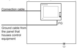
If electric potential difference between the ground points created by it causes malfunctions, lowering the voltage as shown in Remedy 1 below may solve the problem.
