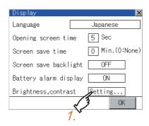
1. Touching the setting items displays the brightness contrast adjustment screen.
