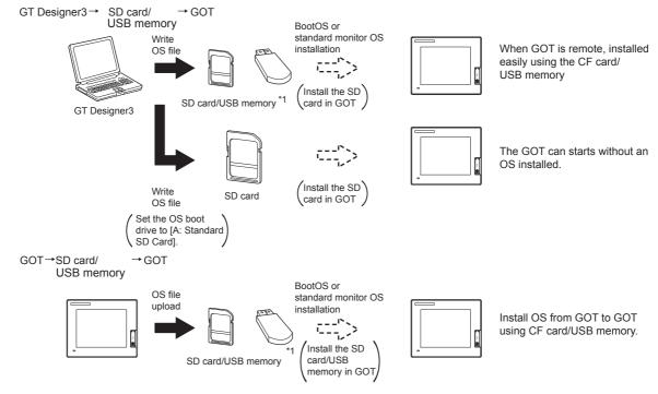
When execute installation with USB memory, standard monitor OS has to be installed in GOT in advance.
