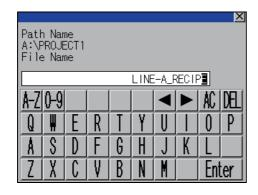
2. Touching [Rename] button displays the screen shown left. Input the file name to be changed. By touching the following button, input text type is changed.
