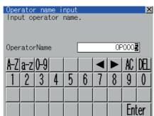
(a) Touch the OperatorName, and then the Operator name input dialog box is displayed. Input an operator name.
