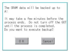
The dialog box shown left appears.Check the description of the dialog box. To back up all data in the SRAM user area, touch the [OK] button.
