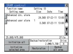
To back up data in the SRAM user area to a drive Select the drive where the data is to be stored, and then touch the [Backup all area] button.
