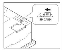
Set the SD card access switch of the GOT to "OFF."
