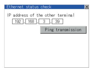
If touch the select button of [IP address of the other terminal], a keyboard is displayed. Enter the IP address of the other terminal with the keyboard.
