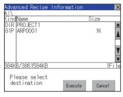
Select the target folder. (Selecting a folder is not needed for outputting directly below the drive.)
