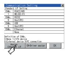
Touch the [Assign Ethernet I/F] button in Communication Setting.
