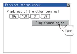
2. If touch the [Ping transmission] button, a ping is sent to the IP address entered in [IP address of the other station].
