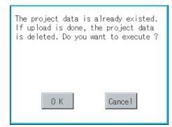
If there is a project data of the same name in the A drive, the screen shown on the left is displayed without starting the upload.
