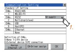
Touch the [5V power supply] button in [Communication Setting].
