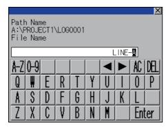
The input key window shown left appears, then input the file name to be created. By touching the following button, input text type is changed.
