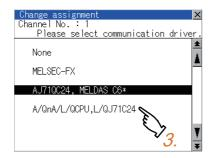
3. As the communication driver ([A/QnA/L/QCPU, L/QJ71C24]) installed in the GOT is displayed, touch it.
