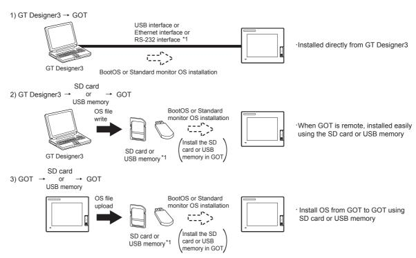
When installing the BootOS and standard monitor OS, standard monitor OS has to be installed in GOT in advance.
