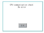
2. When the connecting target confirmation communication ends, its result is notified by dialog box. If the connecting target confirmation communication ends normally, the dialog box notifying of the normal termination mentioned left is displayed. Touching [OK] button after confirming the result returns to [I/O check].
