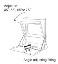
Adjust the mounting angle of GOT with the angle adjusting fitting of the stand.
