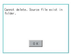
When it cannot be deleted, the dialog box shown at left appears. (Only when deleting folder is executed.)
