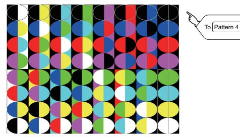
• Pattern 4: Shape check The drawn figures are displayed in order and at regular intervals. If the shape and interval are displayed visually in order, it is normal. Touching the upper right part of the screen returns to the [Display check] screen.
