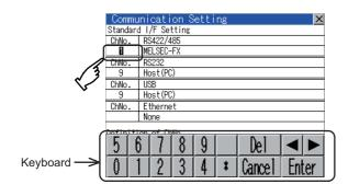
Standard I/F Setting A/QnA/L/QCPU,L/QJ71C24 USB Host(PC) Ethernet None Definition of ChNo. O:None 1–2:FA device 3:External device 9:PC connection CH-Driver assign 0K
