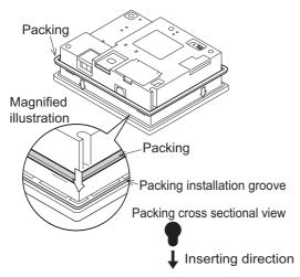
Installing the packing Install packing to the packing installation groove on the back panel of the GOT.
