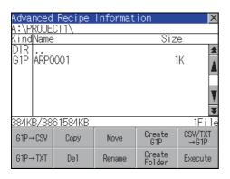
To select the file, touch the check box of CSV file or Unicode text file to be converted to a G1P file.
