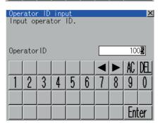
(b) Touch the OperatorID, and then the Operator ID input dialog box is displayed.
