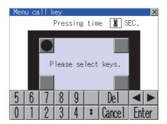
When setting 1 point, specify the time to switch to the utility in case of keeping pressing the key position.
