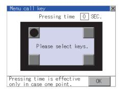
1. Touch or displayed at the 4 corners of the setting screen. The button repeats with every touch. Set the corner to be set to a key position to .
