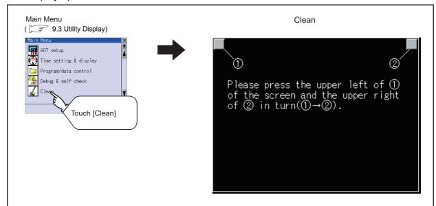
Even if touch points other than the upper left corner and upper right corner of the screen, the GOT does not operates.
