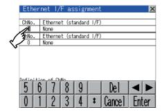
After the screen shown left is displayed, touch the channel number specification menu BOX when changing the channel number.
