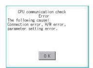
If the dialog box mentioned left is displayed after selecting connecting target confirmation or during CPU communication check, confirm the following.
