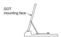
2. Put the GOT into the stand from the stand front side and fix it using the mounting fixtures. For how to mount the GOT, refer to the following.
